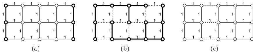
Figure 6. Graph  $G$  and map  $P$  with: (a) in bold, a subgraph  $M$ ; (b) in bold, a MaxSF relative to  $M$  for  $P$  and, in dashed edges, its induced cut, which is not a min-cut; (c) in dashed edges, a min-cut relative to  $M$  for  $P$ .
