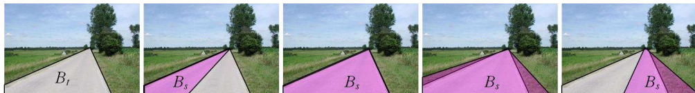
Fig. 14. Illustration of the ‘recall’ concept: the ground truth road segmentation is represented by the gray area in the first image, and the light purple areas in the other images represent the detected road regions. Except for the third image, the ‘recall’ for the other images is smaller than ‘1’.
