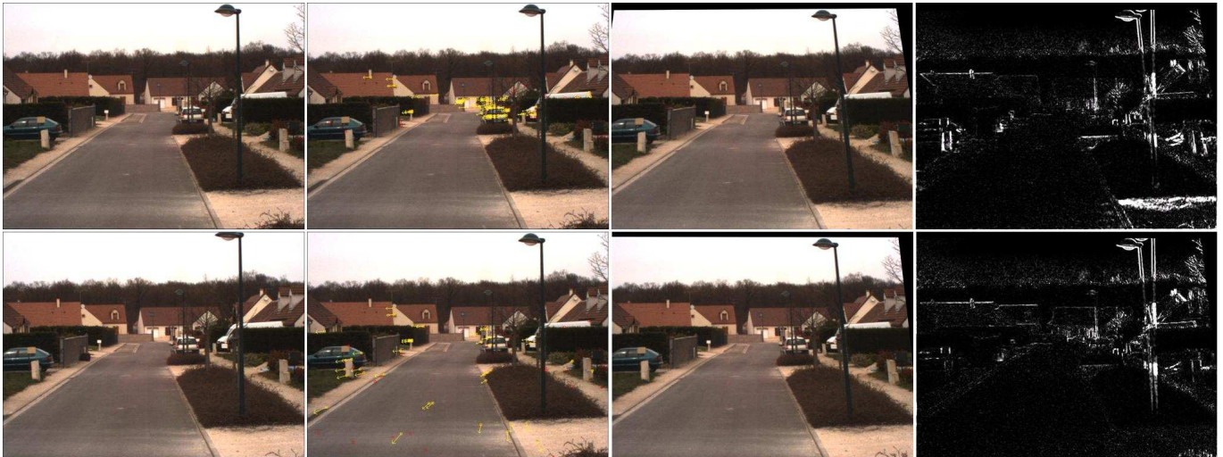
Fig. 3. Examples of alignment based on RANSAC and modified RANSAC (mRANSAC). First column: the reference and target frames. Second column: best inliers obtained from RANSAC and mRANSAC respectively. Third column: the aligned reference frames based on RANSAC and mRANSAC. Fourth column: difference images between the aligned reference frames (by RANSAC and mRANSAC respectively) and the target frames.
