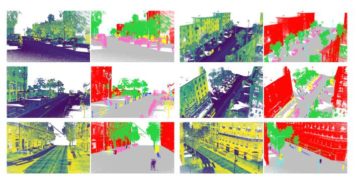
Figure 9: Visual results of our predictions on the test scenes of the NPM3D dataset. The input data is colored according to lidar intensity, from blue (low intensity) to red (high intensity) through green, yellow and orange. Colored, predicted, semantic segments are immediately on the right to lidar images. The segmentation results are obtained with the fusion model (intensity + geometry).
