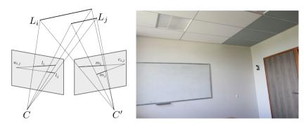
Fig. 1. To register two images, we use the relation between reprojected parallel 3D lines. It allows a more robust and accurate calibration in indoor scenes when points fail to calibrate
