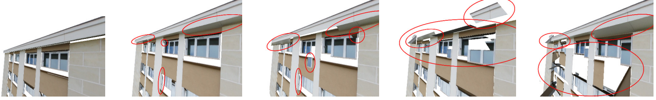
Figure 6: Qualitative comparison of different ablations of our data terms. From left to right: (i) our full model, (ii) Photo+SFM, (iii) Photo only, (iv) Photo+Edge, (v) SFM only. Even though the global pixelwise accuracy may be comparable between different truncated versions of our model (cf. Fig. 5), removing data terms translates into noticeable artifacts which degrade the 3D structure through erroneous depth or even surface orientations. Best viewed in color.
