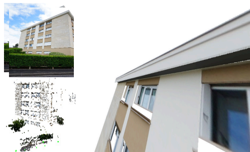
Figure 1: Our method takes a few calibrated images and an SfM point cloud to reconstruct a compact, piecewise-planar mesh aligned with the dominant structure of the scene.
