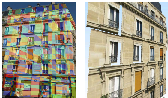
Figure 8: Segments & planes of Haussmannian facade.
