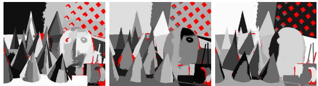
Figure 3. Classification obtained with different precisions. From left to right: precision=1 pixel, 85 planes detected; precision=2 pixels, 44 planes detected; precision=5 pixels, 23 planes detected.
