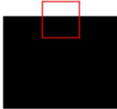
B. Edge Little intensity variation along edge, large variation perpendicular to edge
