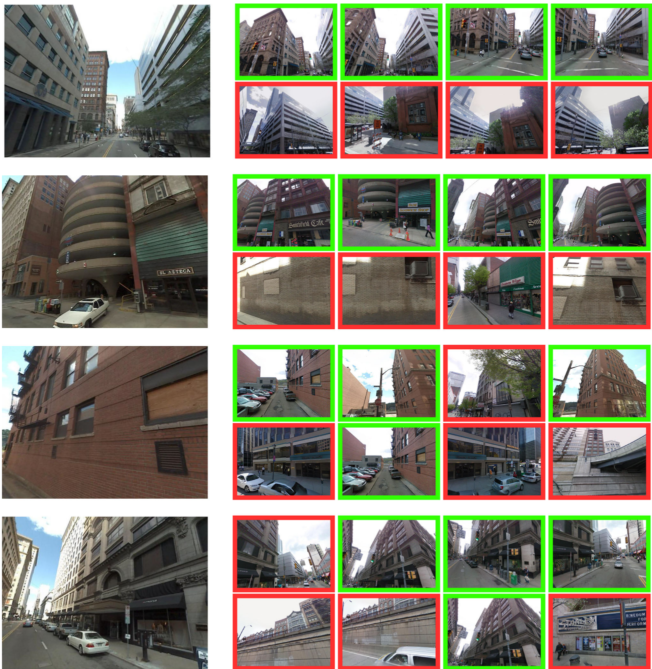
Fig. 8 Examples of correctly and incorrectly localized queries for the learnt bag-of-visual-words representation. Each example shows a query image ( left ) together with correct ( green ) and incorrect ( red ) matches from the database obtained by learnt bag-of-visual-words representation p-val method ( top ) and the standard bag-of-visual-words baseline
