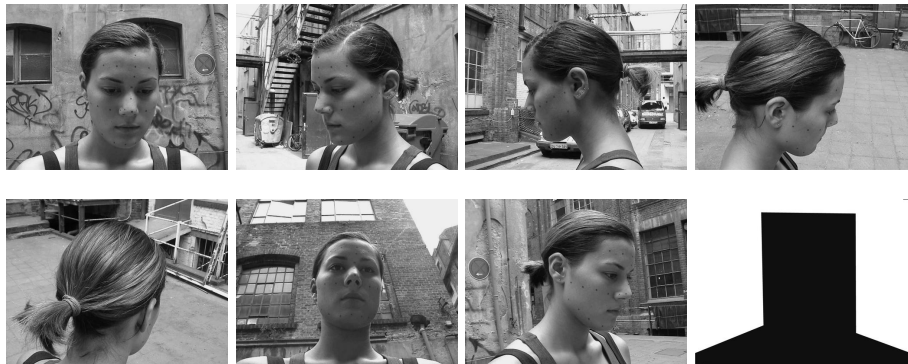
Fig. 4. Contours and stereo-correlation (1): Seven of the twenty images used to recover a human head despite bad lightning condition and few texture information (by courtesy of the RealViZ company). Bottom right: one of the four rough manual detouring used to generate the initial surface.
