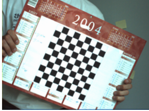
Figure 4: grid used for calibration.
