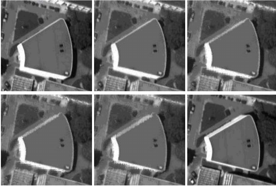
FIG. 2 – MIFFD (4 levels) for an IKONOS satellite stereo pair. From the g image (first from the left), the four reconstructed images from the estimated flow at each level are shown, until the first image f (last one) is approximated.
