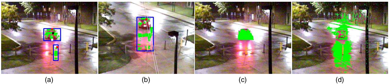
Figure 7: (a) Two-camera initial detection. Here, the specular region was clustered as a separate bounding box. (b) No valid match could be found for the specular region. (c) The specular region successfully removed in the two-camera final detection. (d) Single camera detection in the reference view.
