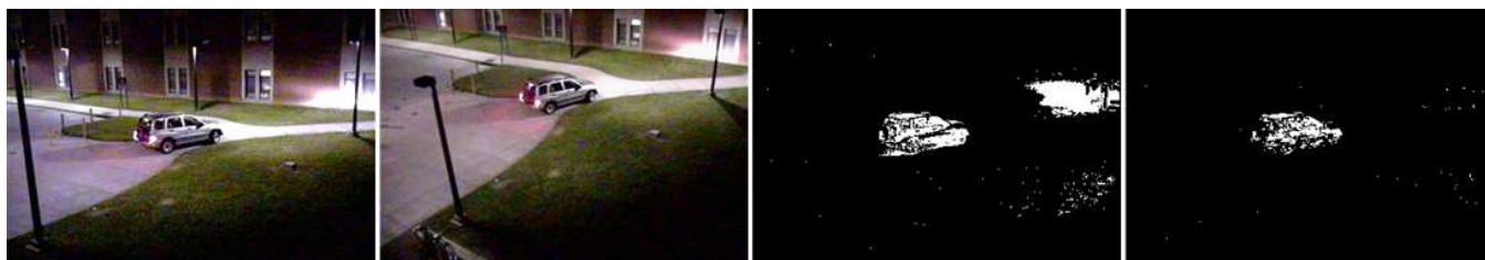
Figure 4: Left to right: reference view, second view, single camera detection and two-camera detection. The usefulness of the proposed sensor configuration is illustrated here. The vehicle's headlight is cast on the wall of the building.
