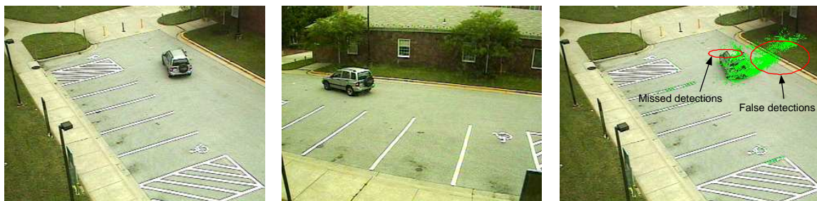
Figure 2: Detection results using the algorithm from [11]. Left to right: reference view, second view and foreground detections. Both missed and false detections are clearly evident.
