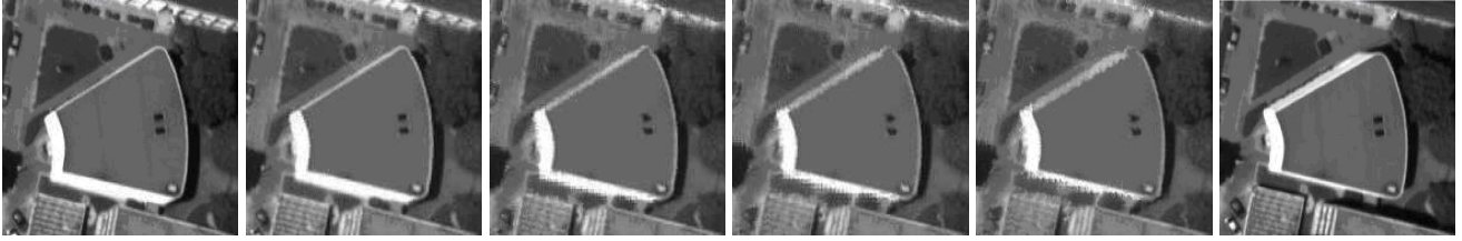
Fig. 4. MIFFD (4 levels) for an IKONOS satellite stereo pair. From the g image (first from the left), the four reconstructed images from the estimated flow at each level are shown, until the first image f (last one) is approximated.
