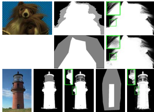
Fig. 1. Sensitivity of Bayesian matting [3] to the trimap. First row: the original image, an accurate trimap and its corresponding alpha. Second row: a coarse trimap and its alpha. Third row: same as rows 1 and 2 for another image.
