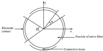
Fig. 2. Transversal section of the nerve-cuff electrode geometry
