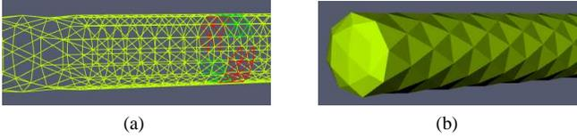
Fig. 3. Zoom of the surface  $S_0$  of the nerve-cuff model. (a) shows that the mesh is finer close to the electrodes. (b) shows that there is a mesh continuity in the boundary of the model.
