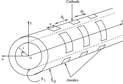
Fig. 1. Schematic design of the nerve-cuff electrode geometry
