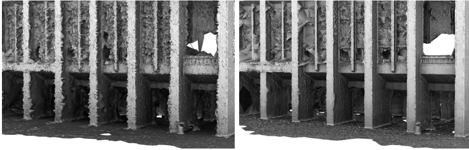
Figure 7.12: Visibility consistent mesh with our GPU sweeping-plane point cloud (left) and PVMS point cloud (right). The PMVS point cloud leads to more accurate initial mesh.
