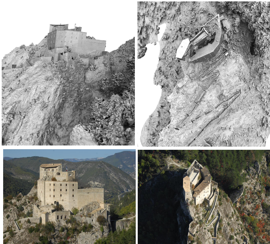
Figure 4.12: Results on Entrevaux data set. Top row: final model of Entrevaux with texture. Two bottom rows: non texture mesh taken from 109 images from a helicopter (© IMAGINE/CSTB), seen in 2 views associated with similar images.
