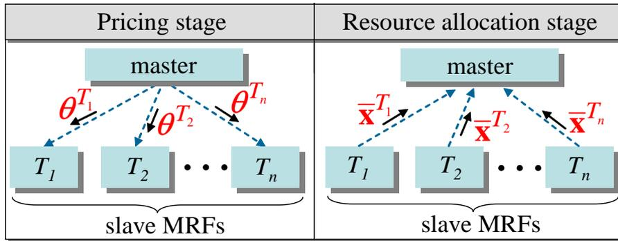
**Fig. 3:** Dual decomposition scheme for MRF optimization **Left:** Based on the current optimal solutions  $\{\bar{\mathbf{x}}^T\}$  (i.e. the current resource allocation), the master assigns new MRF potentials  $\{\boldsymbol{\theta}^T\}$  (i.e. new prices) to the slave MRFs. **Right:** Based on these new potentials, the slave MRFs immediately respond to the master by sending to him new optimal solutions  $\{\bar{\mathbf{x}}^T\}$  (i.e. by readjusting their resource allocation).
