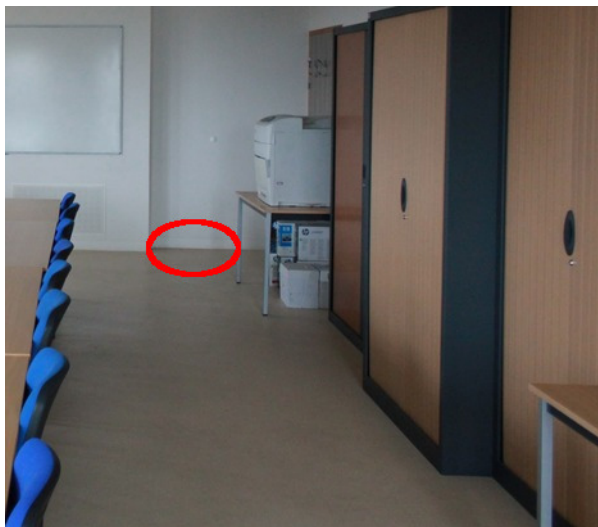
Figure 10: Missing detections of 3D lines in the input: visible edge between floor and wall in a view of the MeetingRoom dataset (left), and extracted lines with Line3D++ where that important edge is missing to recover the floor (right).
