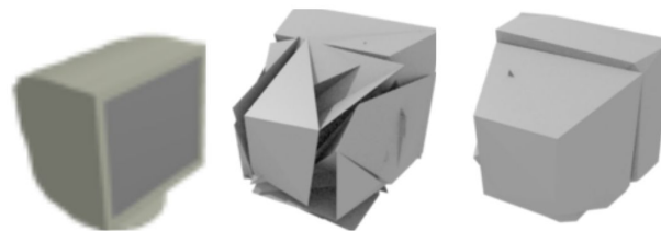
Figure 5. Generation of the back side of a CRT monitor with/without smoothness regularizer. Left: input image. Center: prediction without regularizer. Right: prediction with regularizer.
