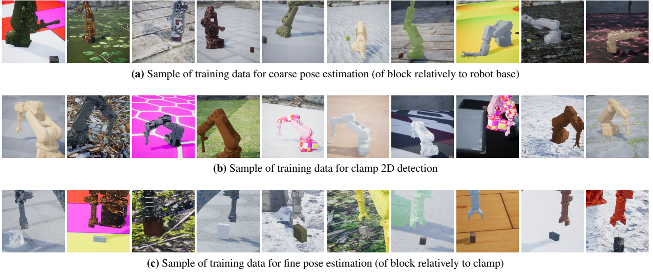
Fig. 4 Our synthetic training dataset covers a large variety of random viewpoints, joint positions, object poses and sizes, as well as texture (for the robot, the block and the environment), making the trained model robust to all of these parameters
