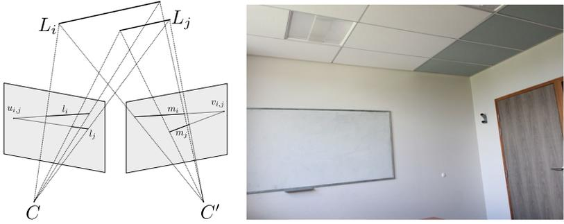
**Fig. 1.** To register two images, we use the relation between reprojected parallel 3D lines. It allows a more robust and accurate calibration in indoor scenes when points fail to calibrate.
