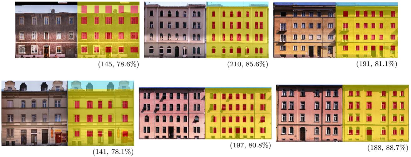
**Fig. 12** Qualitative results on Graz2012 dataset. Image (left) and segmentation using learned grammar  $\mathcal{G}_{cl}$  (right) are shown here along with number of episodes for convergence and segmentation accuracy.
