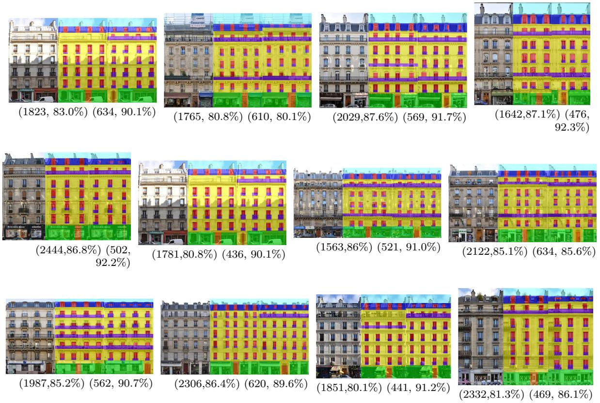
**Fig. 14** Qualitative results on ECP2011 dataset. Image (left) and segmentation using handwritten grammar (center) and learned grammar  $\mathcal{G}_{cl}$  (right) are shown here along with number of episodes for convergence and segmentation accuracy.
