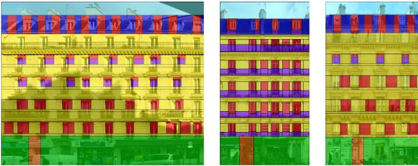
**Fig. 2** Segmentation maps after 5000 iterations of RL parsing [62] with the generic grammar of Table 1.
