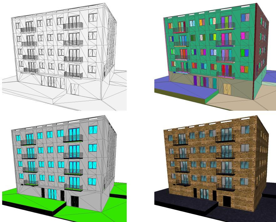
Figure 16: LcD building with, from upper left to lower right, model without semantization, after polygon extraction, after semantization and with texture.
