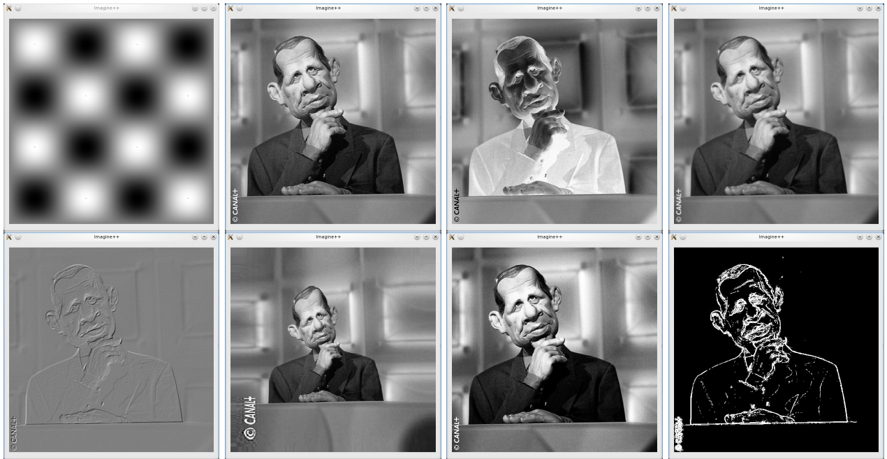
FIGURE 1 – Two images and various processing on the second one (negative, blur, relief, deformation, contrast and edges).
