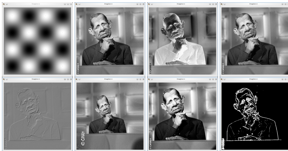
Figure A.7: Two images and various processing on the second one (negative, blur, relief, deformation, contrast and edges).
