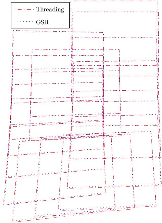
Figure 5. Overlay of frame borders found with Threading versus GSH after BA. The borders of the reference frames (upper right) align well. At the other extremity (lower left) discrepancies of several pixels can be seen.
