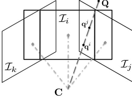
Figure 1. Sweep of images with a static center of projection  $C$  (no parallax): the real 3D point  $Q$  projects to  $q^i$  in image  $\mathcal{I}_i$  and its corresponding point  $q^j$  in  $\mathcal{I}_j$ , but is not visible in  $\mathcal{I}_k$ .
