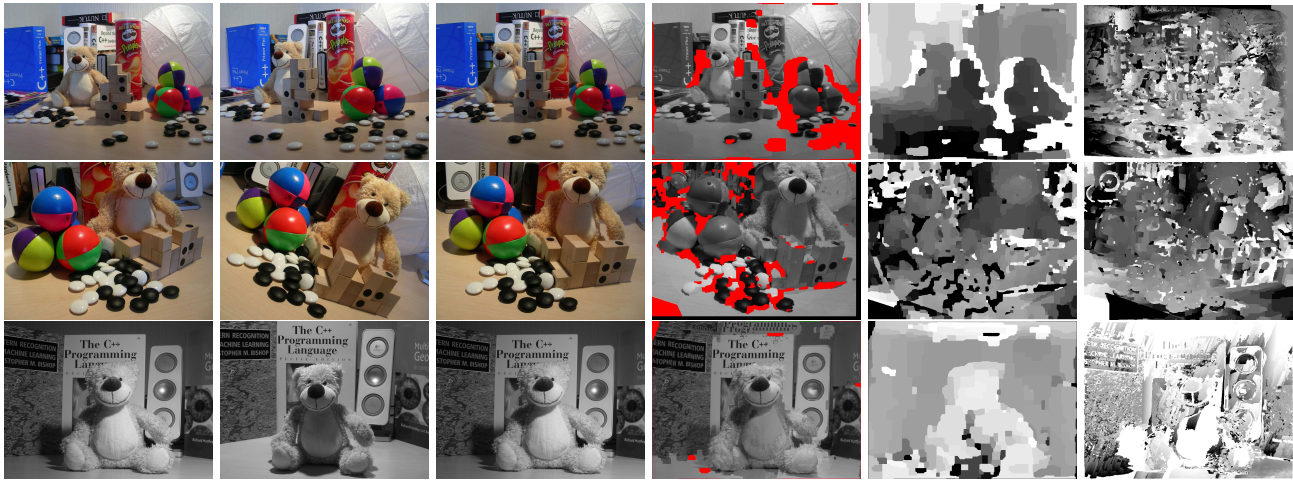
Figure 8: Depth maps and resynthesized images. In each row, the first two images are the inputs to our stereo-matcher. The third one is not used to compute the depth but only to validate the quality of the fourth one, which is synthesized from the first two using the DAISY depth map shown in fifth position. The final image is the depth map computed using correlation. The occluded areas are overlaid in red in the synthesized images and they're black in the depth-maps.
