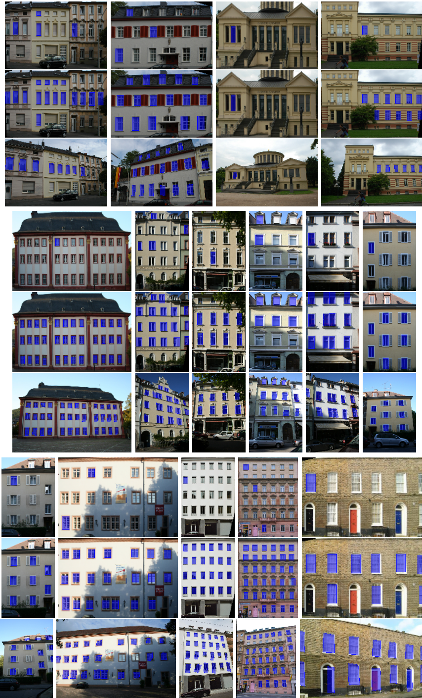
Fig. 5: Window detection results on the eTRIMS dataset (2/2): input quadrilaterals, detections on rectified images, and detections on non-rectified images.
