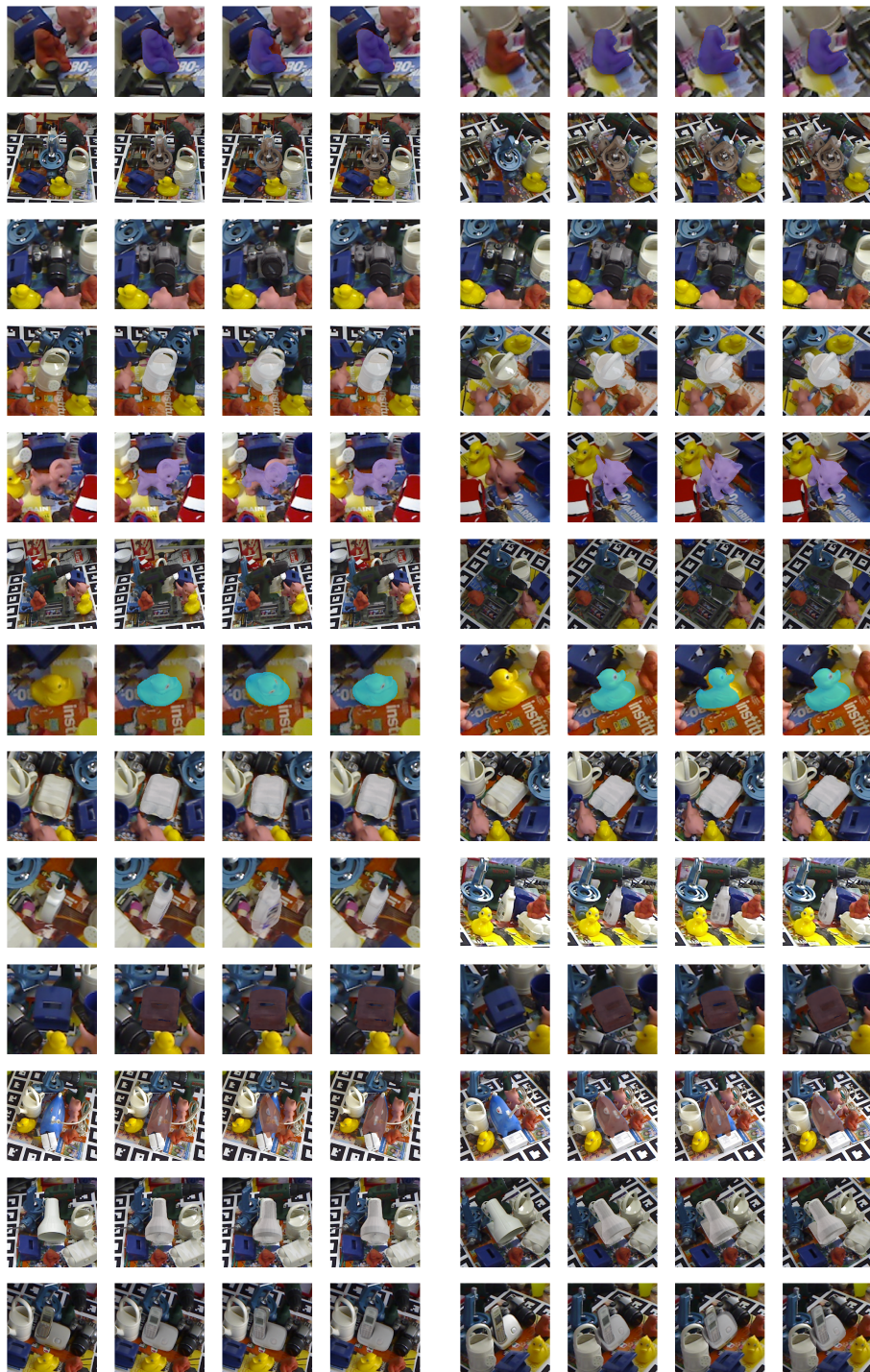
Figure 1: Visual results of object pose estimation on LINEMOD [1]. For each sample, the four columns from left to right represent: the input image, the correct shape and orientation, our initial estimate and the final estimate after refining our initialization with DeepIM [2].
