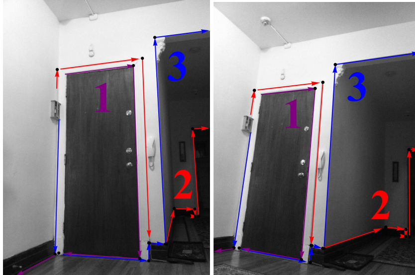
Fig. 5. Three extracted chains. The added segments must preserve the global orientation of the chain (clockwise or counterclockwise) and its continuity.
