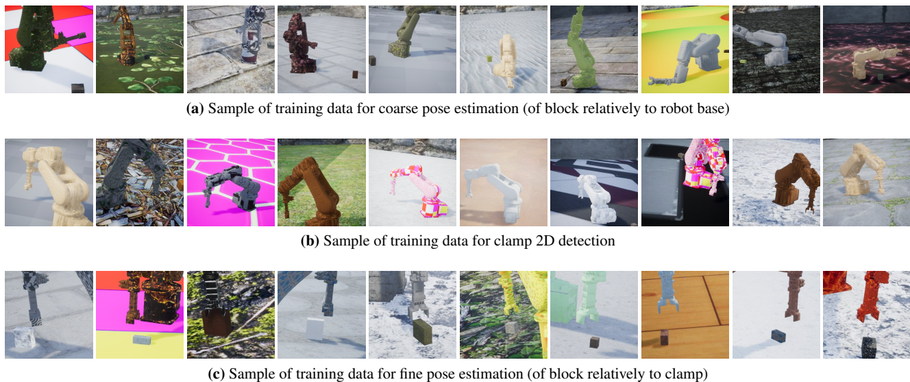
Fig. 4 Our synthetic training dataset covers a large variety of random viewpoints, joint positions, object poses and sizes, as well as texture (for the robot, the block and the environment), making the trained model robust to all of these parameters
