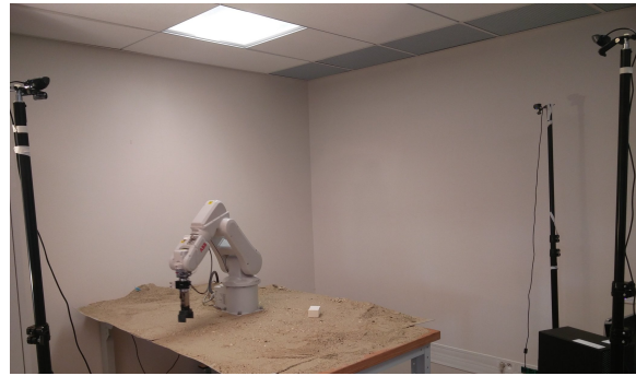
Fig. 5 Acquisition of real images to create our test dataset, with 3 cameras at arbitrary and varying positions
