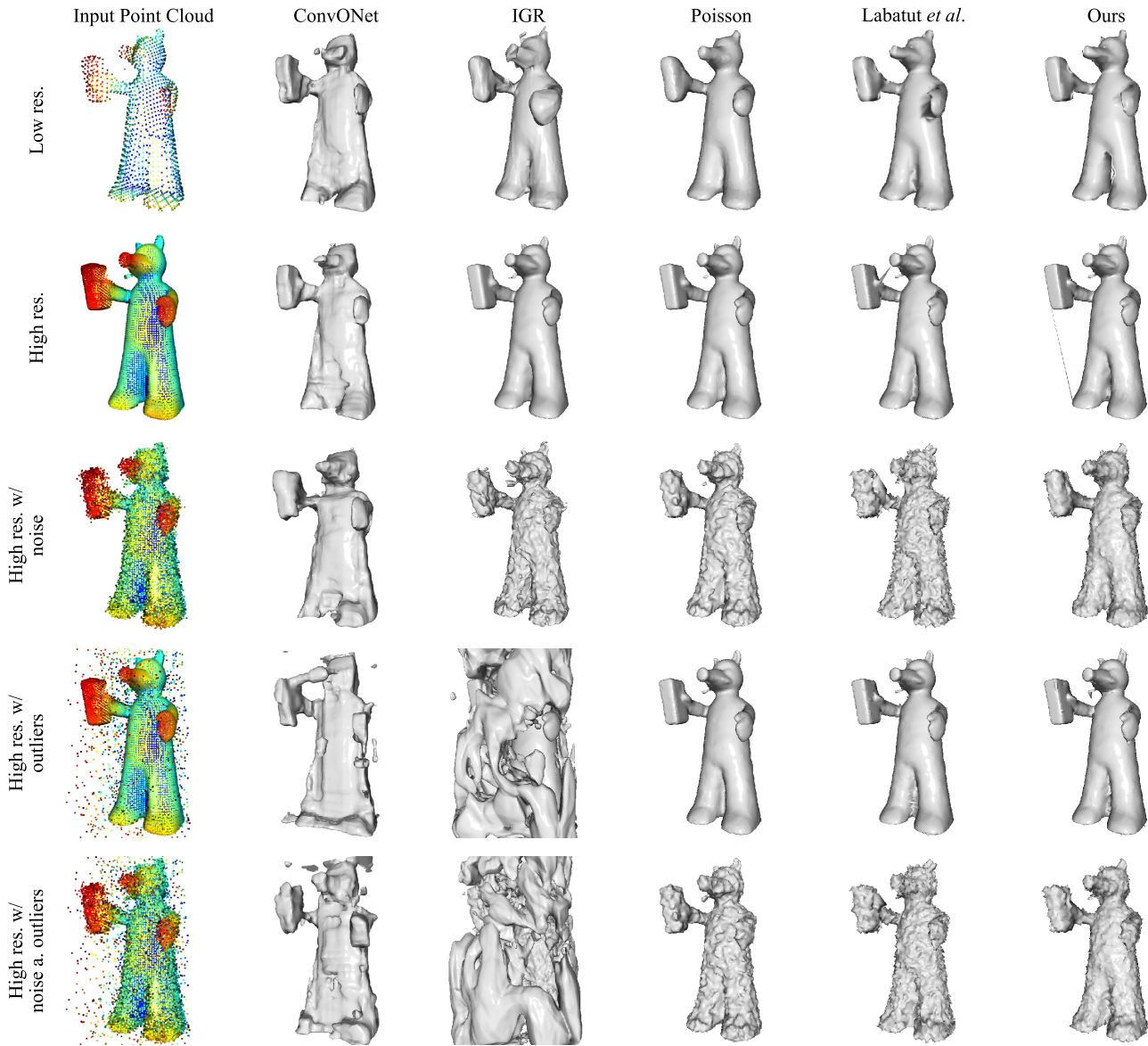
Figure 12: Reconstruction of the Quasimoto object in the surface reconstruction benchmark of Berger et al. [BLN*13]. We show the input point clouds in column 1. ConvONet [PNM*20] (column 2) does not generalize well to the unseen new shape. IGR [GYH*20] (column 3) is not able to filter outliers in the scan. The Screened Poisson [KH13] algorithm (column 4) does not reconstruct the sharp features well. The reconstructions of Labatut et al. [LPK09] (column 5) and ours (column 6) are visually similar for the defect-free cases. Both methods produce small artifacts in the high resolution case: between the book and nose for Labatut et al. [LPK09] and between the book and left foot for ours. Both methods are very robust against outliers.
