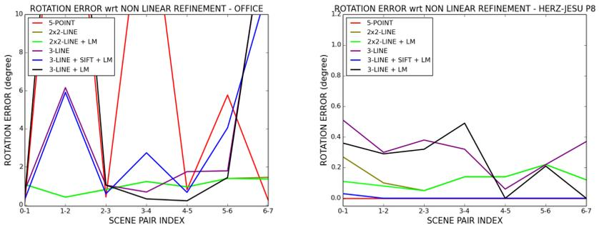
**Fig. 6.** Rotation error for image pairs in datasets *Office* (left) and Strecha’s Herz-Jesu-P8 (right). Reported methods do not use their final refinement stage (Levenberg-Marquardt, LM) unless otherwise mentioned. The curve for “ $2 \times 2$ -lines + LM” is often hidden by the “ $2 \times 2$ -line” curve.
