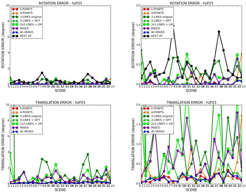
Fig. 25. Pose estimation error for each image pair. Top: rotation error. Bottom: translation error. Left: graph in range 0-10°. Right: zoomed graph in range 0-2°.
