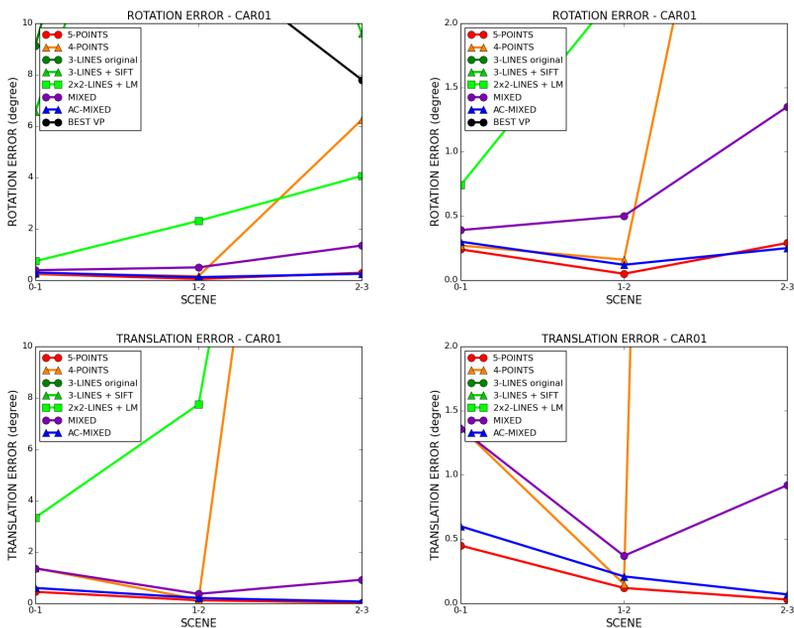
Fig. 13. Pose estimation error for each image pair. Top: rotation error. Bottom: translation error. Left: graph in range 0-10°. Right: zoomed graph in range 0-2°.
