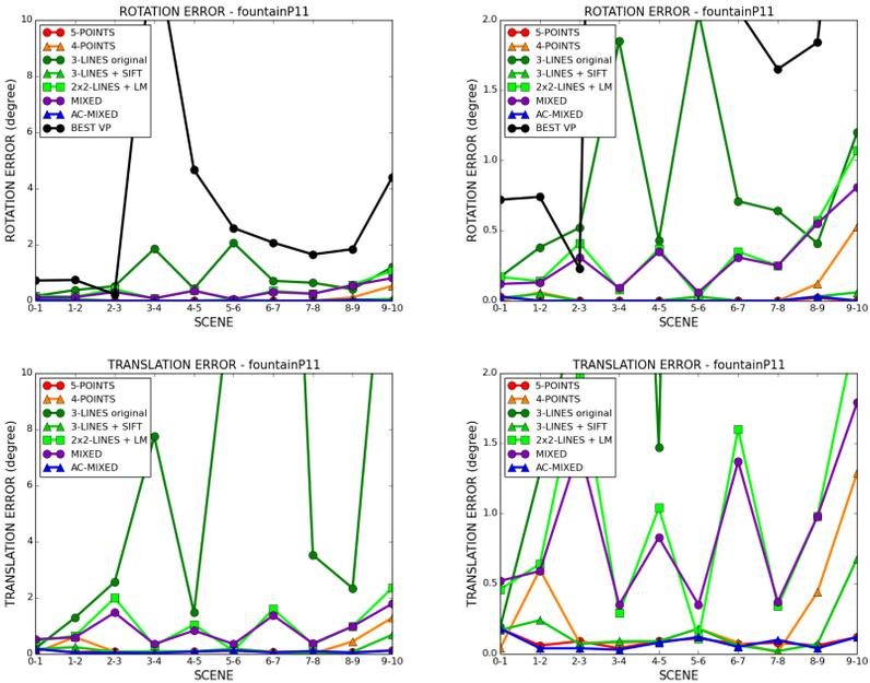
Fig. 21. Pose estimation error for each image pair. Top: rotation error. Bottom: translation error. Left: graph in range 0-10°. Right: zoomed graph in range 0-2°.
