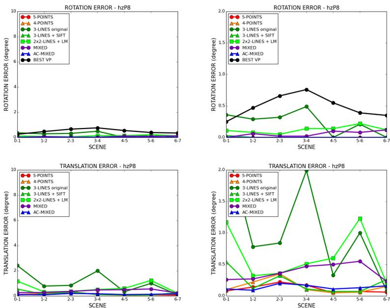
Fig. 23. Pose estimation error for each image pair. Top: rotation error. Bottom: translation error. Left: graph in range 0-10°. Right: zoomed graph in range 0-2°.
