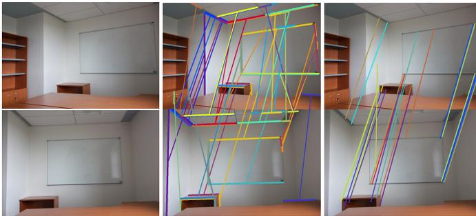
**Fig. 8.** Example of images from *Office*, line matches and points matches.
